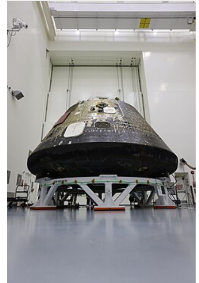
Vehicles like the Orion's Crew Module 6 are featured with thermal protection system, allowing theoretical reusability of the capsules.
