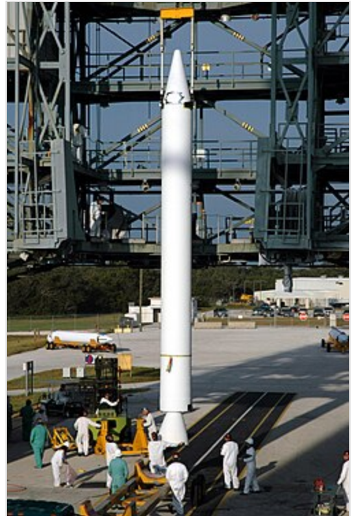
A GEM-40 strap-on booster for a Delta II launch vehicle.
