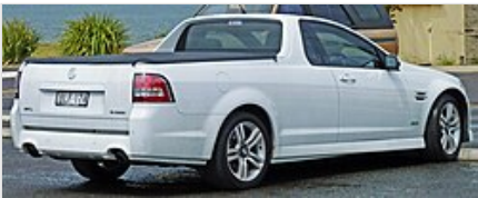
The Ute ( pictured ) is built upon the Caprice's 3,009 mm (118.5 in) wheelbase. ✂
