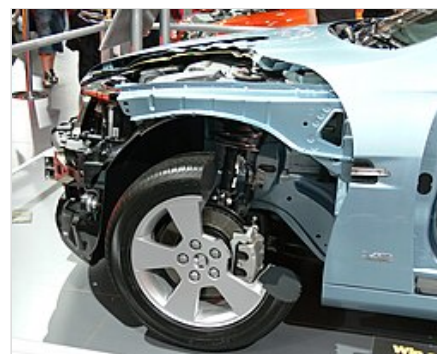
Internal cut-away revealing the VE Calais (MY07 pictured) engine bay and suspension setup
